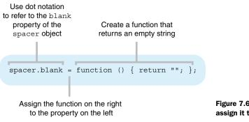
Figure 7.6 Create a function and assign it to an object property
