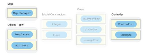
Figure 20.9 The modules for The Crypt with new or updated modules highlighted
