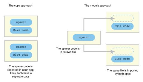
Figure 13.2 Moving spacer into a module allows the same single file to be used in many projects.
