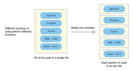
Figure 13.1 Breaking one large program into modules
