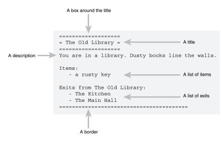
Figure 9.4 The elements shown when a Place object is displayed on the console.
